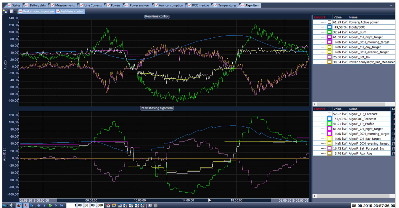
Figure 20 Storage real time daily diagram, upper window are measured values, forecasted values are presented in the lower part
