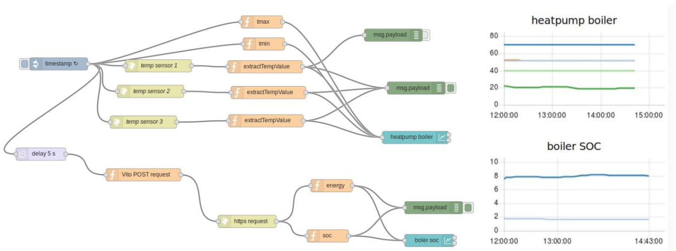
Figure 6. A quick test program written in Node-Red to test the API for temperature data.
