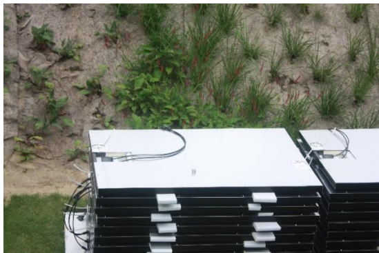
Figure 4: Pile of PVT panels ready for installation. An aluminium radiator of the type of the back of a fridge is glued to the back of a standard PV panel. Consequently, an insulation panel that can resist high temperatures is put on top of it and a closing aluminium shield is attached to finish. The part around the junction box is left open, to allow maintenance and free cooling.
