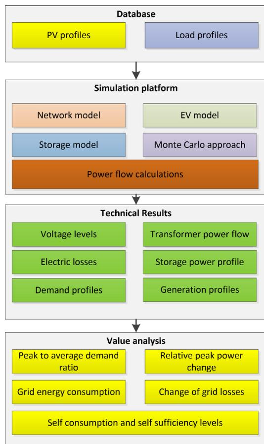
Figure 1: Simulation and analysis process
