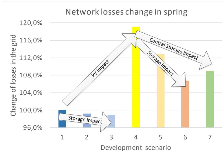
Figure 3: Losses in the network comparison
