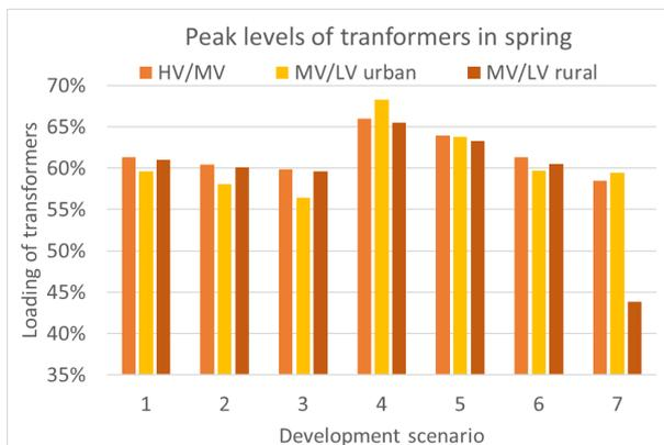
Figure 4: Peak loading levels of transformer in spring
